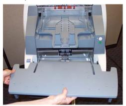
The manual feeder has two locations for the side guides. Depending on the size of the documents you are scanning:
