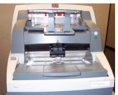
2. Place the manual feeder on top of the elevator tray using the slots in the manual feeder to align with the side guides. Position the manual feeder to the fully seated position.
