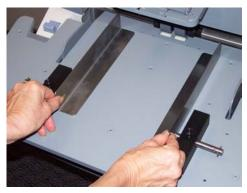
6. Tighten the screws on both side guides to secure them in place.
