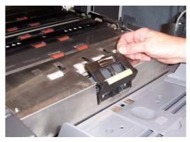
To install the new separation roller:
