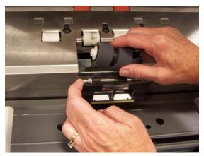
4. Push the separation roller holder back in place and close the pod.
