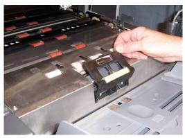
3. Insert the new separation roller. Be sure to line up the slots on the separation roller with the holders.
