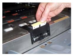
3. Install the new pre-separation pad. Be sure it snaps into place.
