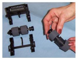
5. Install each new tire by gently stretching it over the core.
