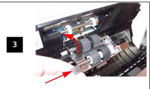
Insert new roller and rotate roller assembly up.
