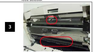
Ending sensor, skew sensors and starting sensor.
