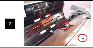
Paper sensor, waiting sensor and double feed detector
