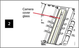
Locate the camera glass cover between and below the LED lamps. Clean it with a dry swab. **Do not use solvents when cleaning the camera glass.**
