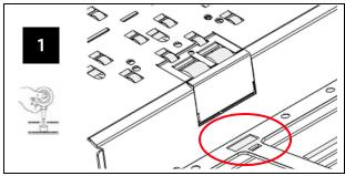
Use the blower brush to clean all 7 sensors. The feed sensor is shown above.
