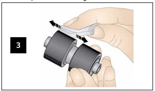
Scrub the roller tires in a side-to-side motion with a roller cleaning pad and re-install the roller. Reinstall the pick roller when finished.
