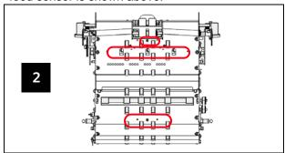
Clean the gap sensors, page entry sensors and pass thru sensor.
