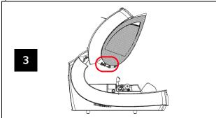
Clean the exit sensor which is located on the transport toward the back of the scanner.
