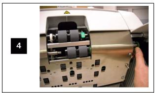
Remove the drive roller by pushing the roller to the right. Hold the drive roller in place and slide it off the shaft. Gently release the drive roller shaft back into position.
