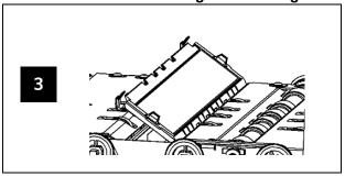
Reinsert the imaging guide into the scanner.
