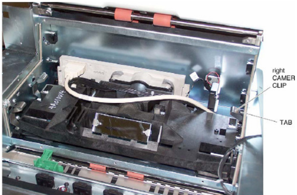
Figure 13 Remove scan module by removing 3 clips, Scan Module PCB is attached.
