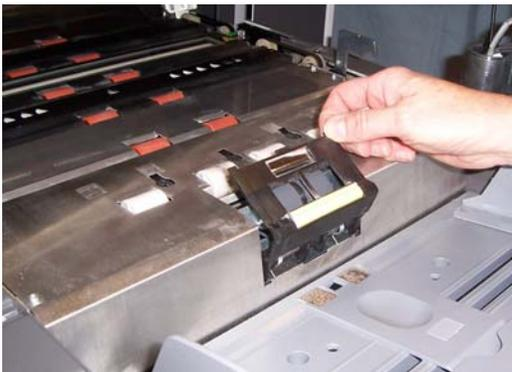
To install the new separation roller:
