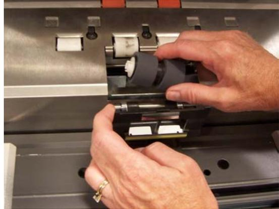
4. Push the separation roller holder back in place and close the pod.
