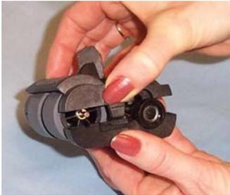
9. Press the upper and lower housings together until they snap into place.
