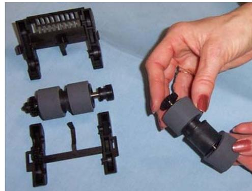
5. Install each new tire by gently stretching it over the core.
