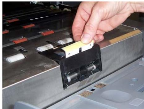
3. Install the new pre-separation pad. Be sure it snaps into place.
