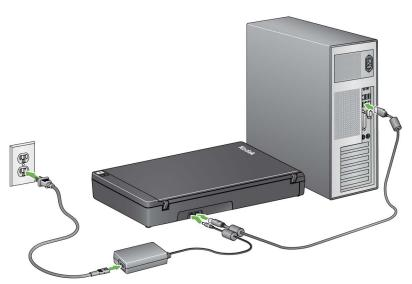
5. Connect the other end of the USB cable to an open USB port on your PC.
