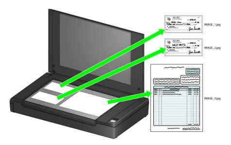
You can scan the documents using the Start/Resume button on the flatbed or scanner; or use the desired application.
