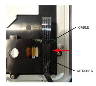
[3] Gently release the CABLE from the RETAINER; it is taped to the RETAINER.
