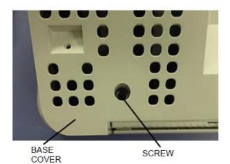
[1] Remove the SCREW from the bottom of the BASE COVER.
