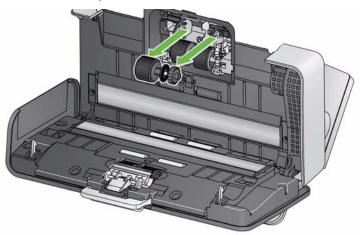
3. Rotate the lower feed roller so the pin is positioned with the open slot, then lift the roller out of position.
