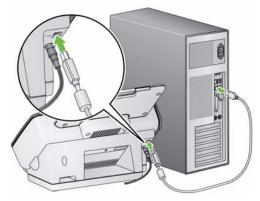
4. Attach the USB cable to the scanner USB port, located on the back of the scanner.
