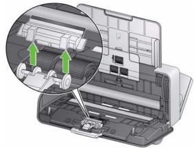
2. Remove the separation roller.
